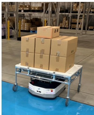
Automated guided robot (introduced on an experimental basis)
